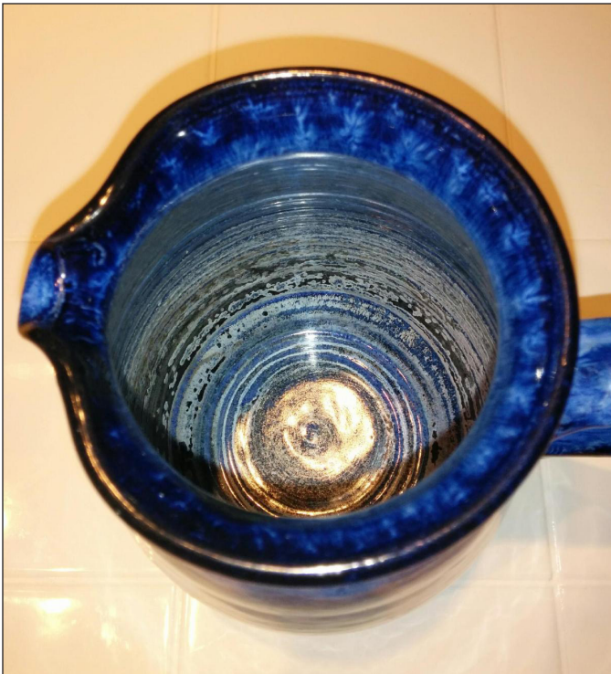
Figure 1. The inside of the jug showing erosions of the inner surface.
